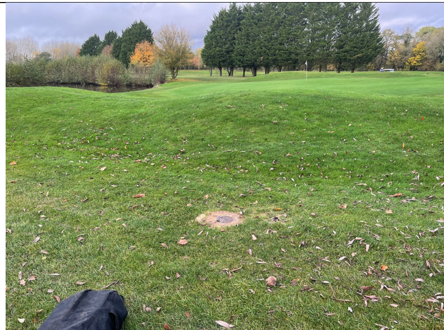
Photo 4. Photo showing greens areas of raised/mounded ground (reinstated borehole in foreground of photograph)
