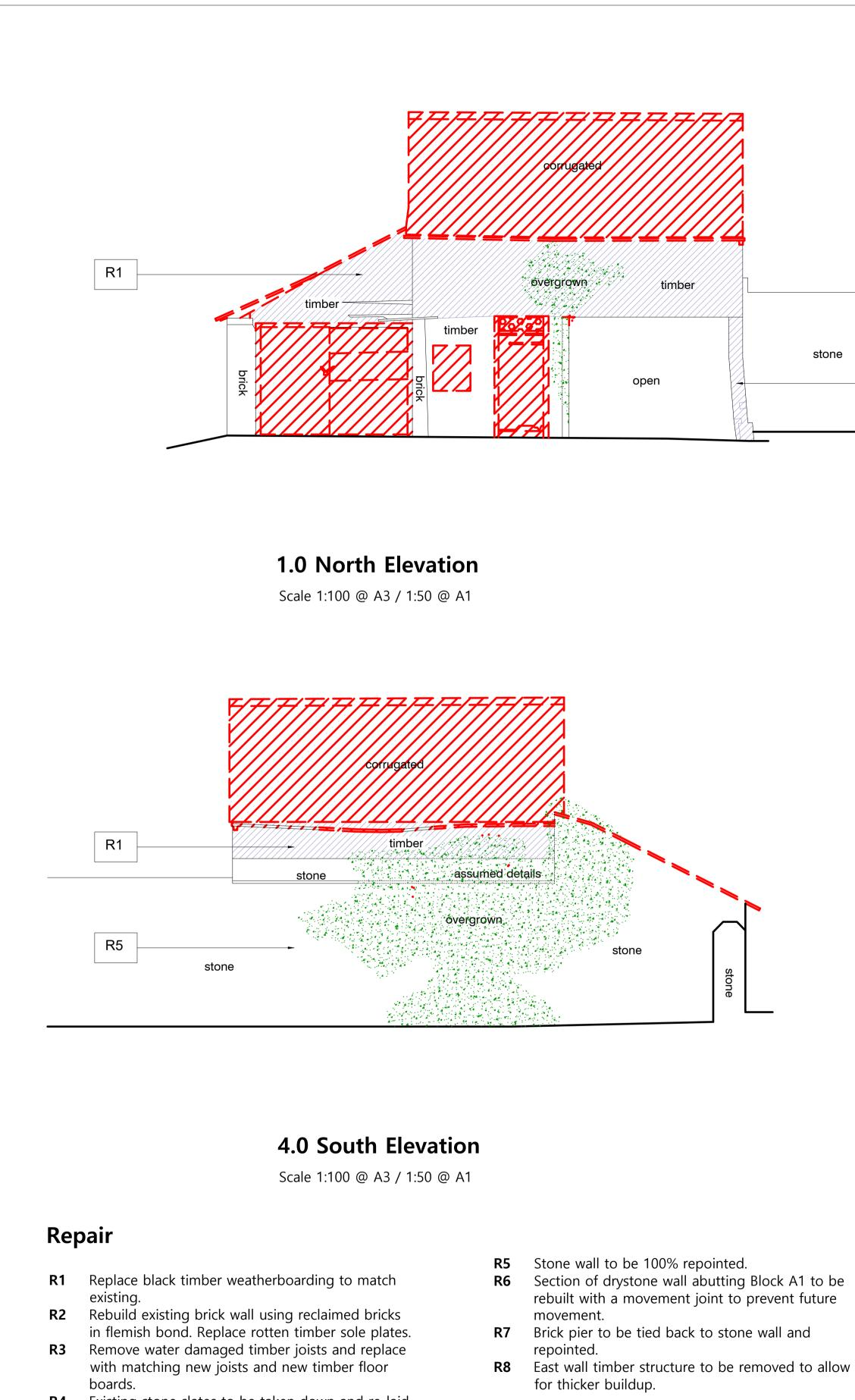
**R4** Existing stone slates to be taken down and re-laid with adequate lead flashing.
