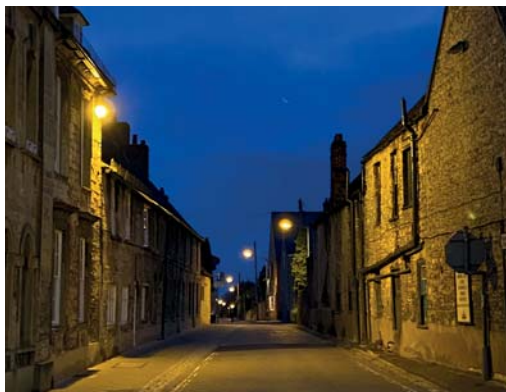
HENSINGTON - NIGHT High pressure sodium street light (at ~7m) Illuminance: 70 lux
