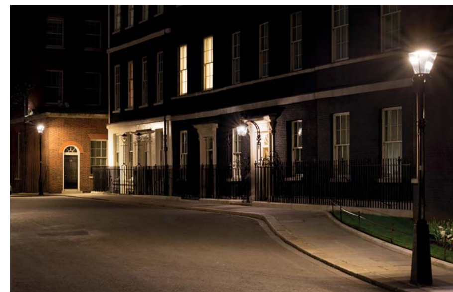
DIMMABLE LED STREET LIGHTS WITH CONTROLLED DOWNWARD LIGHT DISTRIBUTION.
