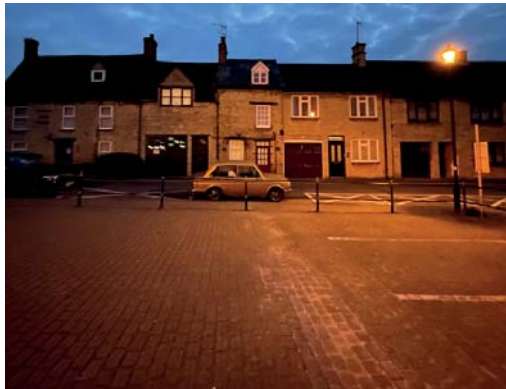
UNION ST - NIGHT High pressure sodium street light (at ~4.5m) Illuminance: 25 lux
