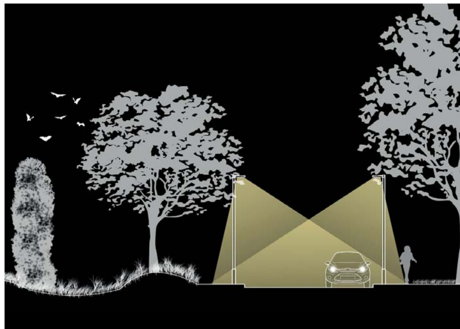
SKETCH CROSS SECTION SHOWING PROPOSED HEDGEROW WHICH CREATES A DARK COMMUTING ROUTE FOR BATS
