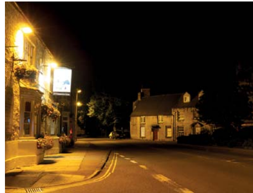
OXFORD ST / HIGH ST - NIGHT Wall-mounted high pressure sodium floodlights (at~4.5m) - Illuminance: 100 lux
