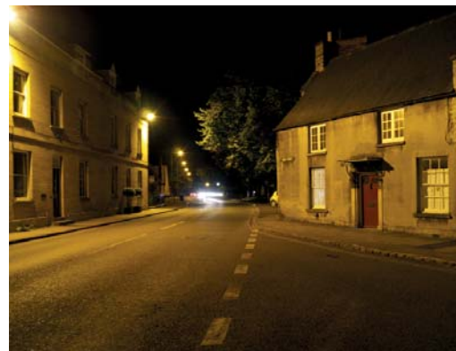
OXFORD ST / HIGH ST - NIGHT Wall-mounted high pressure sodium floodlights (at~7m) - Illuminance: 95 lux
