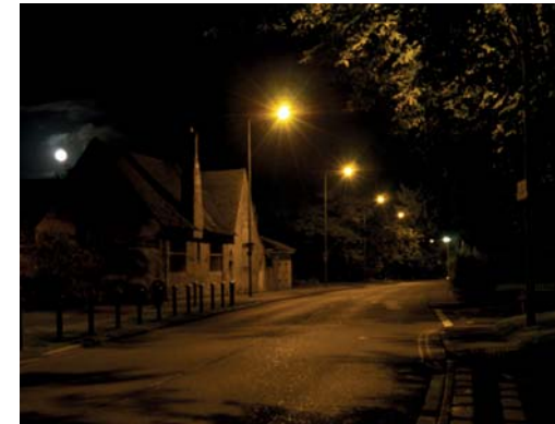
OXFORD RD (A44) - NIGHT High pressure sodium street light (~10m) Illuminance: 12 lux
