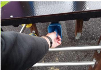
**Finding:** The item fails to meet the requirements of BS EN 1176 Part 1 4.2.7.2 for head and neck entrapment in the frame
