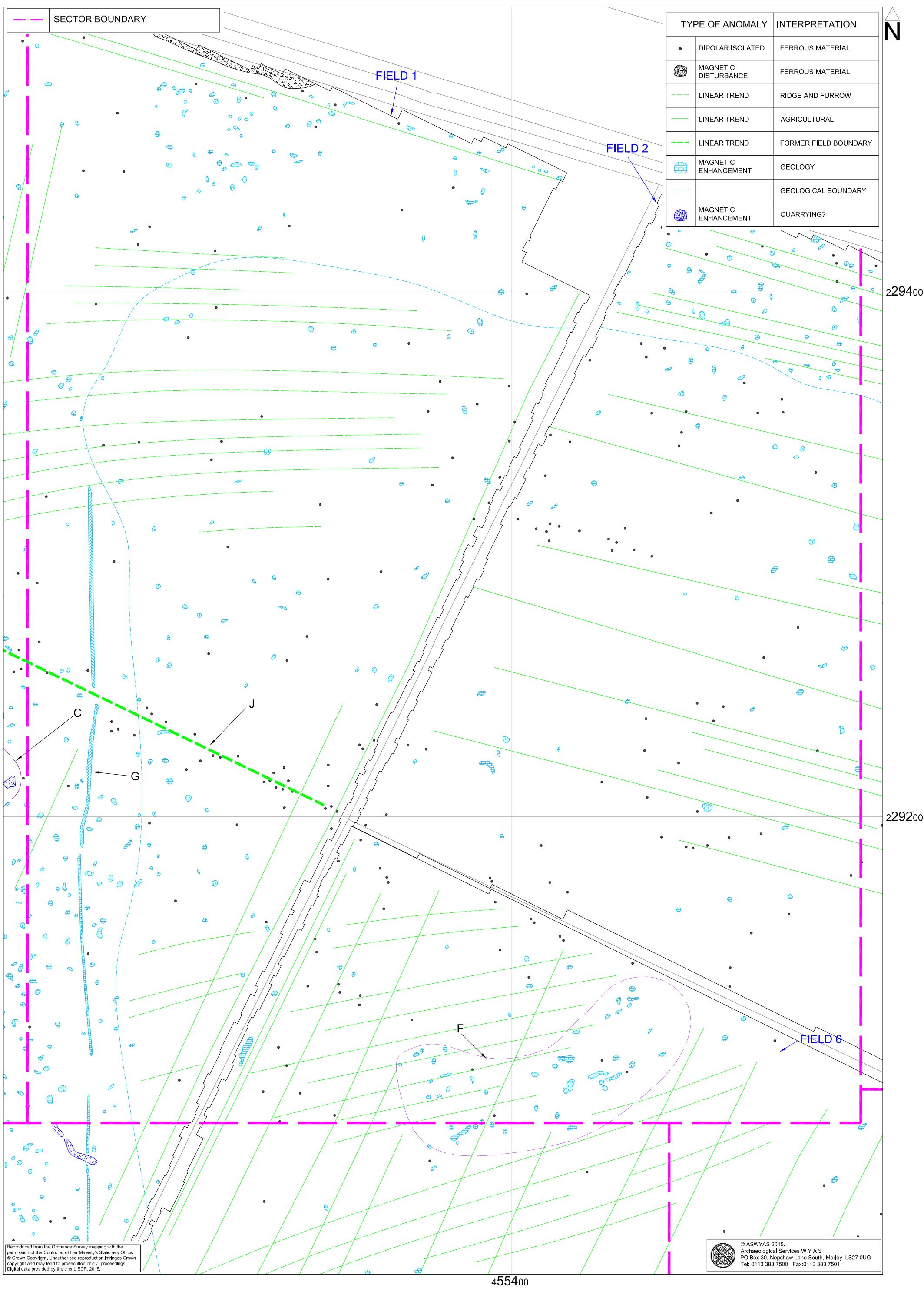
Fig. 10. Interpretation of magnetometer data; Sector 2 (1:1250 @ A3)
