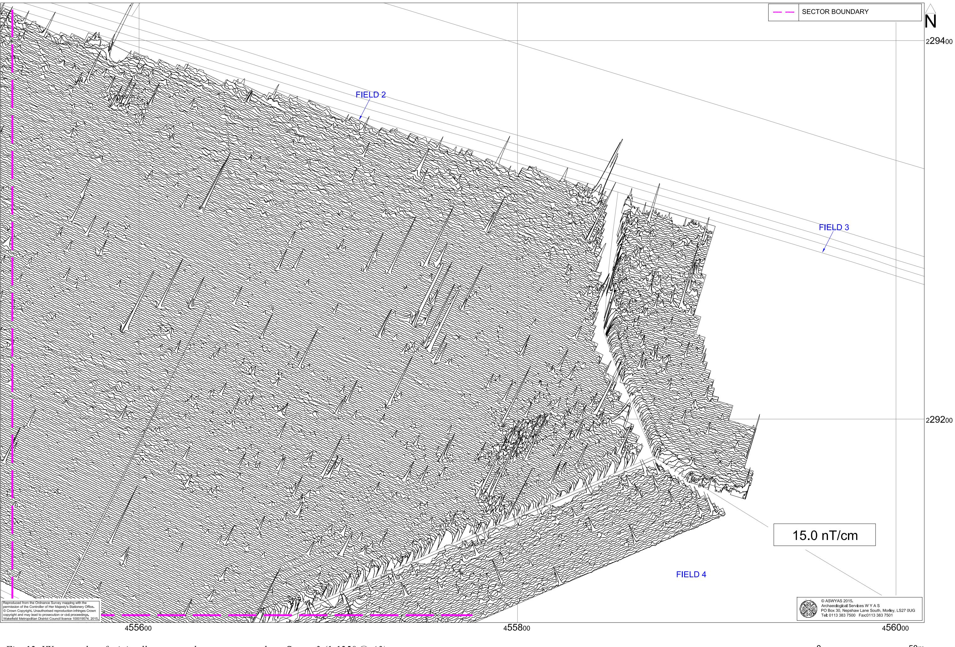
Fig. 12. XY trace plot of minimally processed magnetometer data; Sector 3 (1:1250 @ A3)
