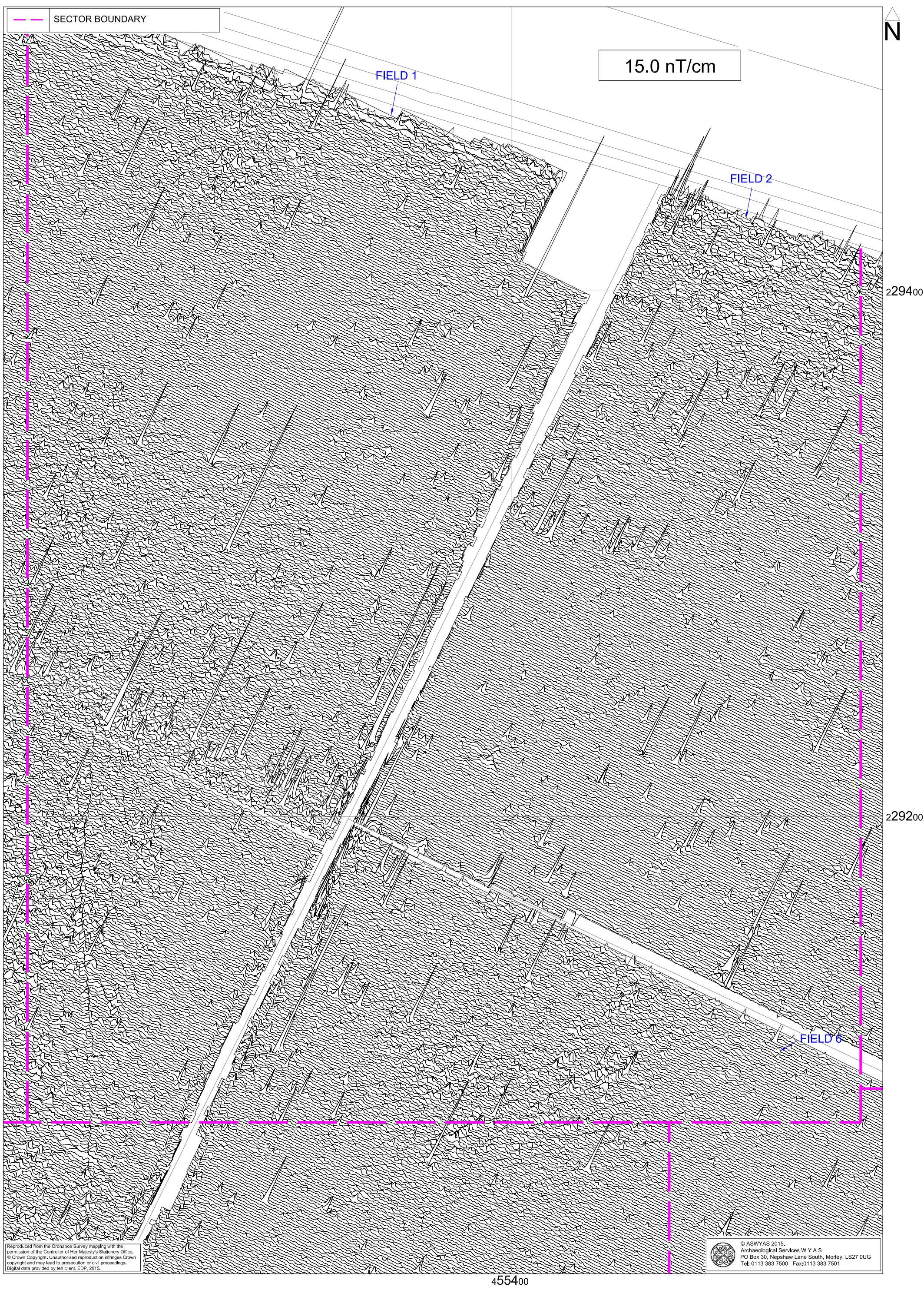
Fig. 9. XY trace plot of minimally processed magnetometer data; Sector 2 (1:1250 @ A3)
