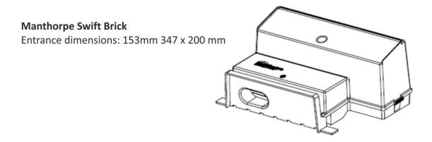
The Swift Brick should be located high within the gable wall of the property, ideally at 5 metres high and above and over the level of the insulation zone. Where possible, install in locations that are unlikely to receive large amounts of direct sunlight during the hottest times of the day, ideal places include below the overhang of the verge and barge board.
