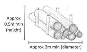
Log piles are designed to provide sheltering opportunities for a range of fauna including reptiles, amphibians and invertebrates. Dimensions should measure a minimum of approximately 2m in diameter x 0.5m height. Refugia can be created from wood or brash piles, and should ideally be positioned across a site in areas of suitable terrestrial habitat.
