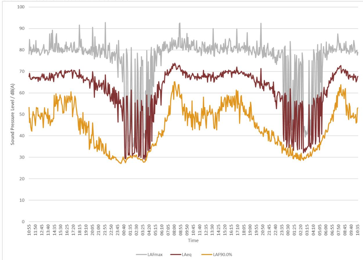
From the measured road traffic noise data, we have determined the following free-field octave band design 'daytime' and 'night-time' equivalent noise levels at the monitoring location:
