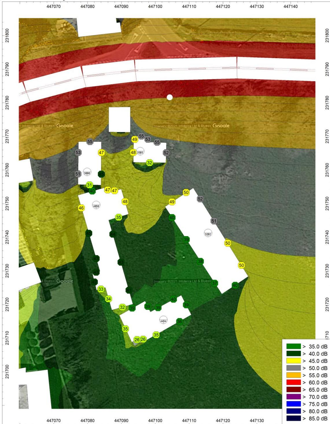
Figure 4. Predicted  $L_{Aeq}$  8 hour dB
