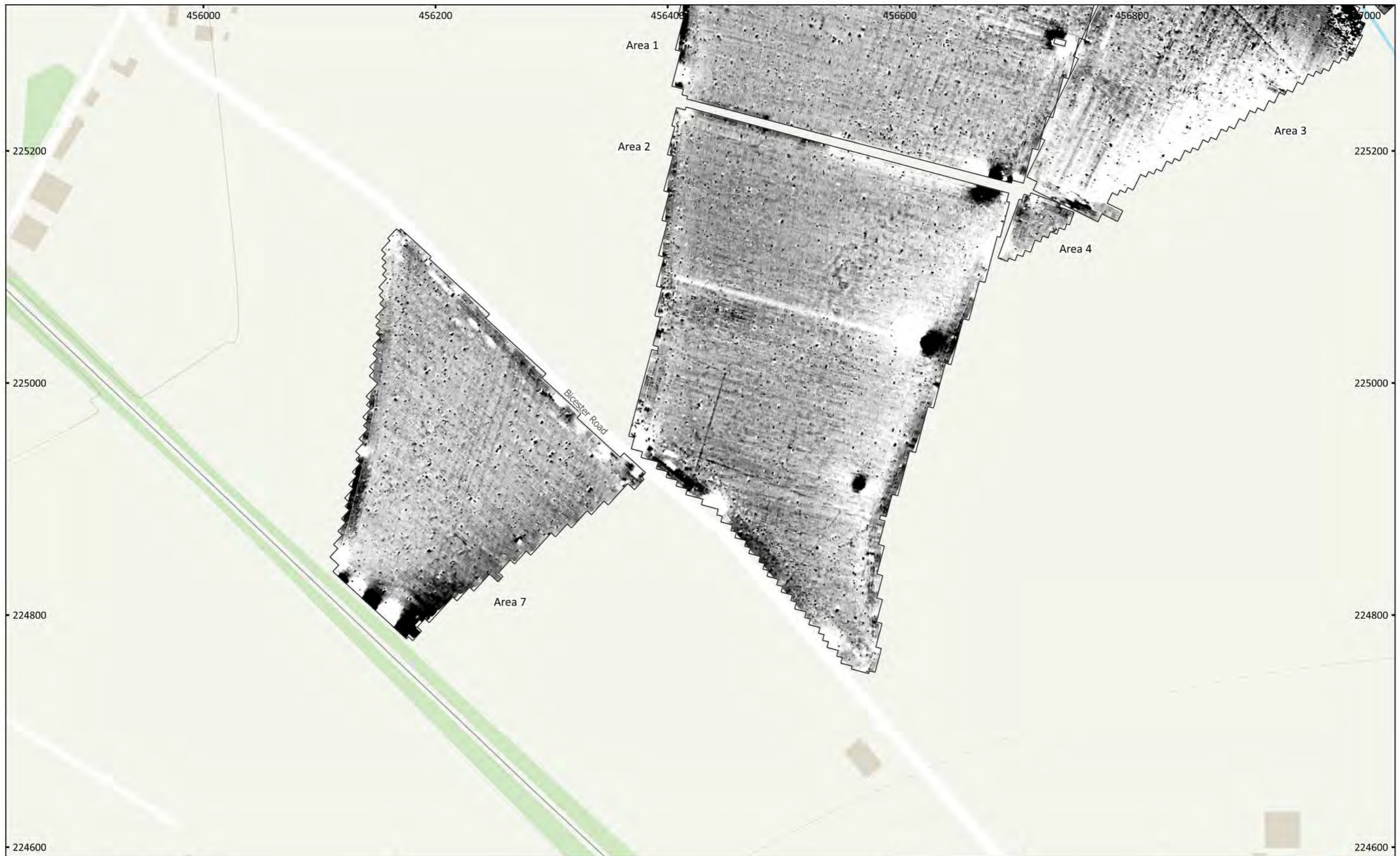
MSSP1197- Land South of Bucknell, Bicester Figure 5 - Magnetic Total Field (Lower Sensor) (South) 1:3,000 @ A3 Copyright Magnitude Surveys Ltd 2022 Contains Ordnance Survey data © Crown Copyright and database right 2022
