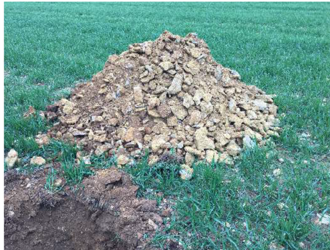
Photo 14: Arisings from trial pit IT07.
