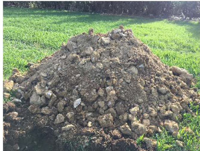
Photo 10: Arisings from trial pit IT05.
