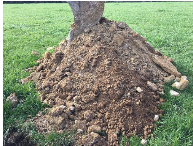
Photo 24: Arisings from trial pit IT12.
