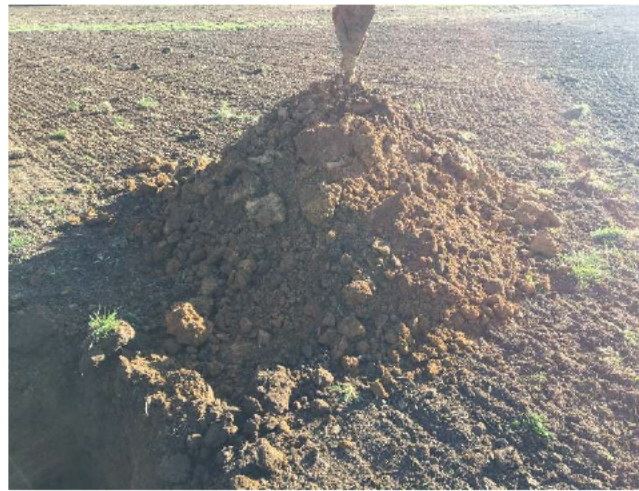
Photo 6: Arisings from trial pit IT03.
