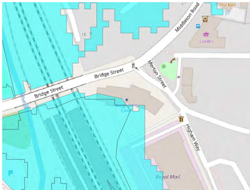
Figure 3: Site location relative to flood zone 2, an area with a 1 in 100yr to 1 in 1000yr annual probability of flooding in any one year (Source: EA online flood data).
