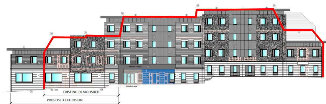
Figure 18: Proposed front elevation of the hotel, red line indicates the existing building outline
