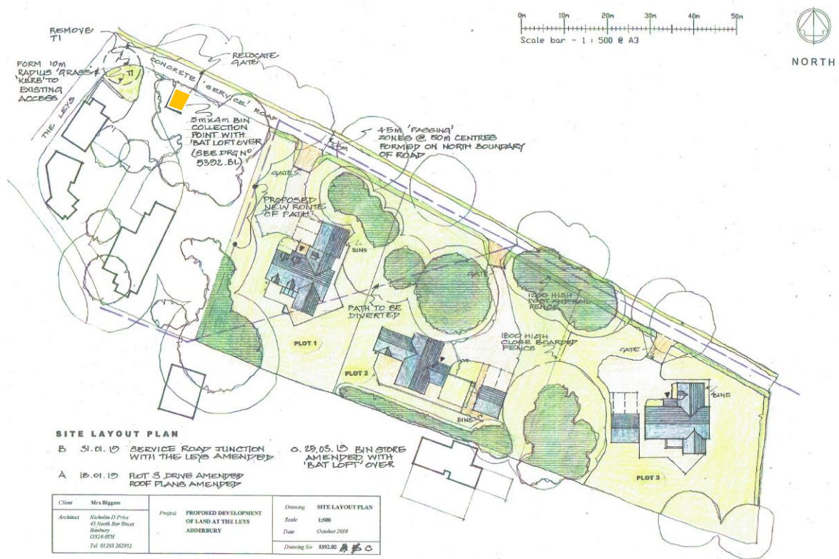
Figure 5 – Permanent replacement bat loft (in orange) for BLE located in loft above bin store
