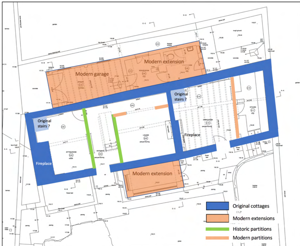
Fig. 25, Interpretation of plan development at ground floor ©SJB Surveying
