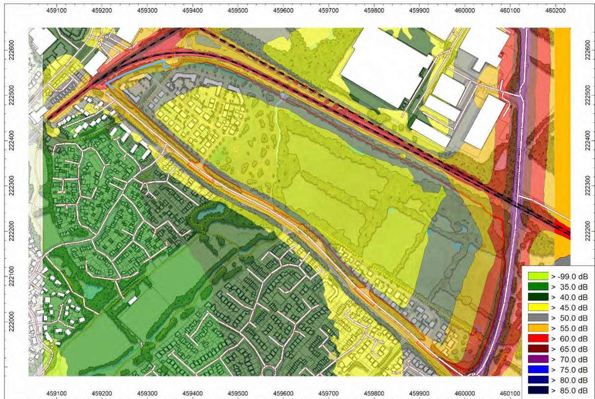
Figure 4: Road and rail noise levels across the site (night time)
