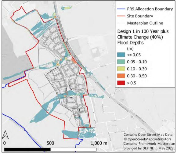
Figure 5-14: Modelled 100-year plus 40% Climate Change Post-developed Flood Depths
