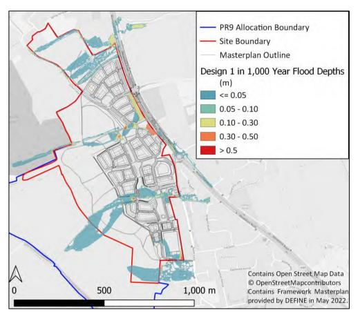
Figure 5-15: Modelled 1 in 1,000 year Post-developed Flood Depths
