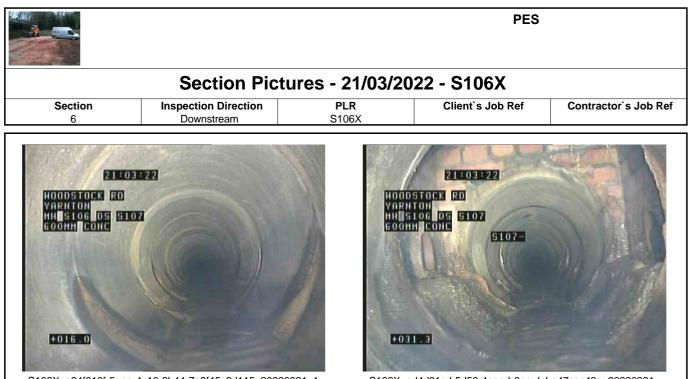
S106X\_a94f010f-5eee-4c10-8b44-7a9f45c6d115\_20220321\_1 50731\_528.jpg, 00:01:35, 16.00 m Attached deposits, encrustation at joint from 3 o'clock to 5 o'clock, 5% cross-sectional area loss, start
