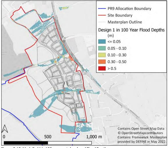
Figure 5-13: Modelled 1 in 100 year post-developed Flood Depths
