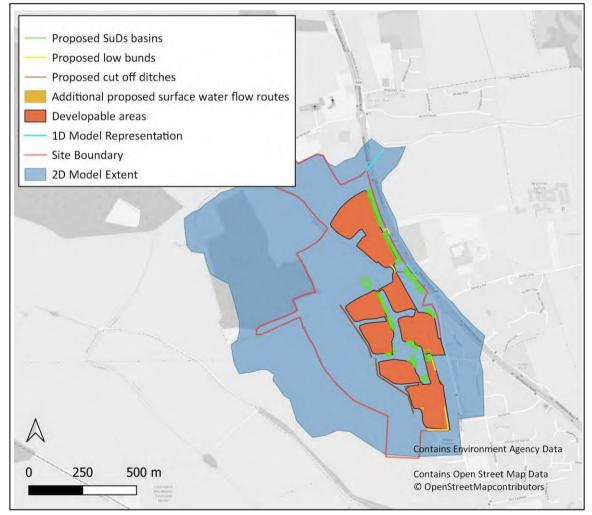
Figure 5-11: Proposed Developable Areas, Attenuation Features and Cut-Off Ditches
