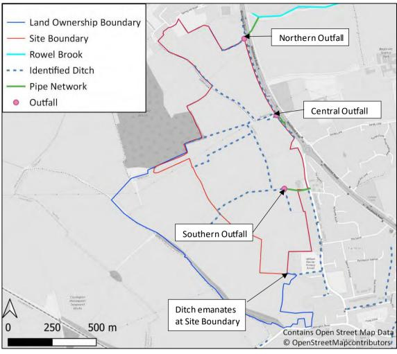
Figure 3-5 – Identified Existing Surface Water Network
