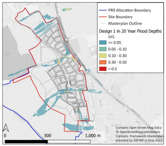
Figure 5-12: Modelled 1 in 20-year post-developed Flood Depths
