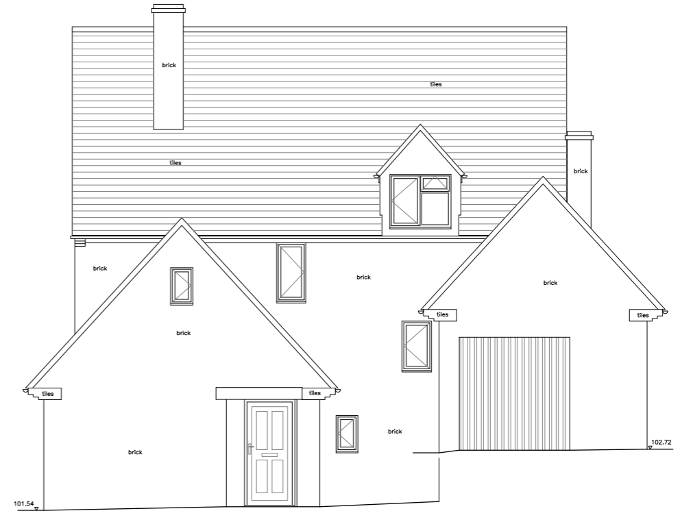
East Elevation 1:100 at A3
