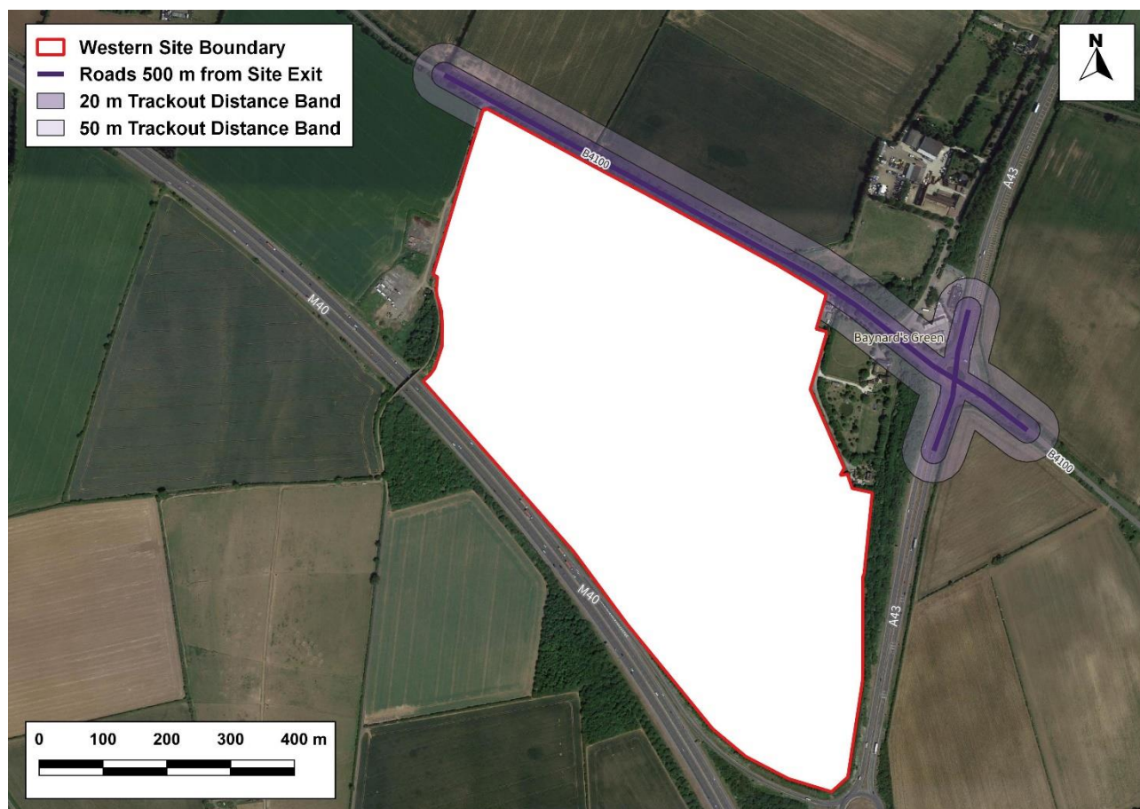
Figure 9.7: 20m and 50m Distance Bands around Roads within 500m of Western Site
