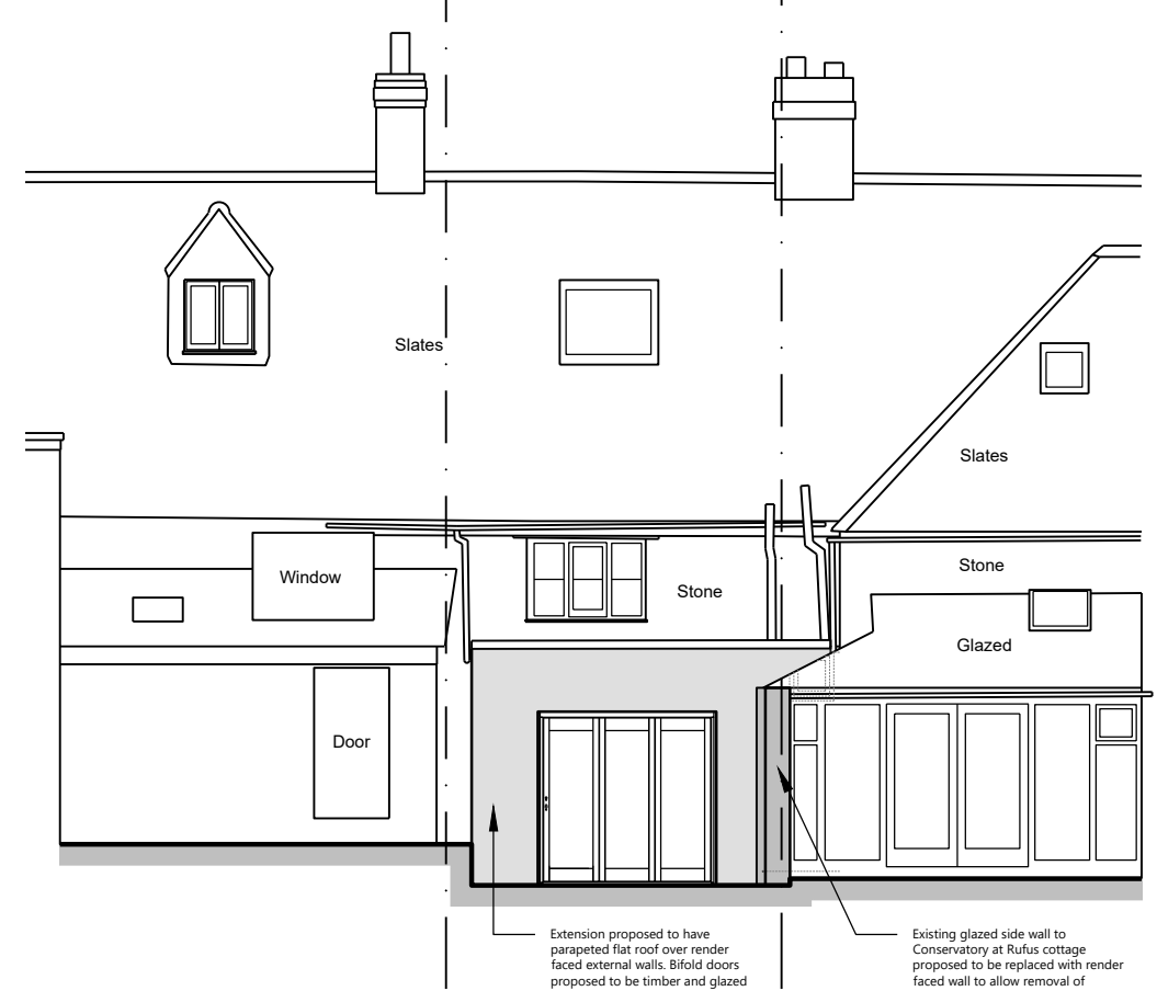
Proposed North Elevation Scale: 1:100
