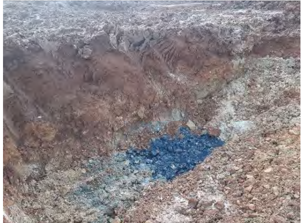
03.02.21 – Hydrocarbon impacted gravel evident by black colouration
