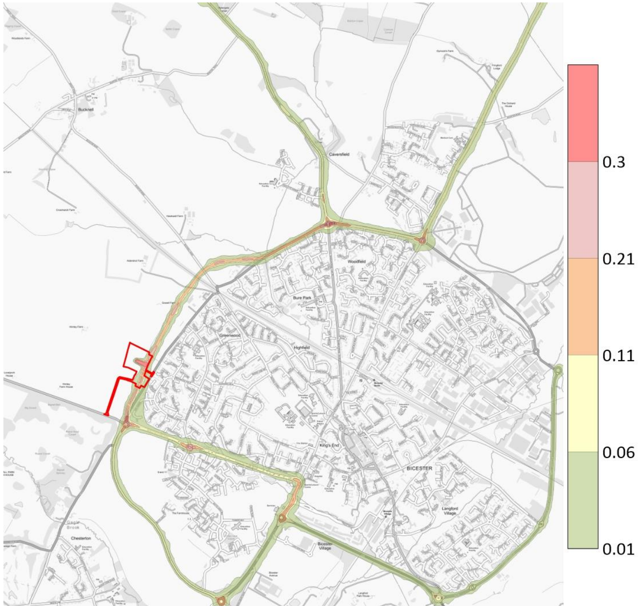
Figure 6-3. Annual Average Long-Term Nitrogen Dioxide (NO 2 ) Contribution from Proposed Development (µg/m 3 ) During the Operational Phase
