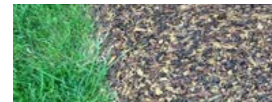
BOUND RUBBER MULCH SAFETY SURFACE
