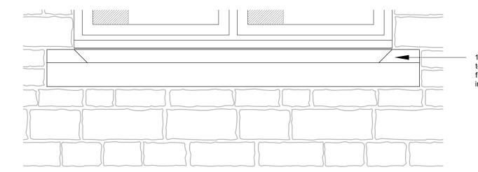
140mm deep Stone cill to project 50mm from finished wall face. Cill to incorporate drip rebate
