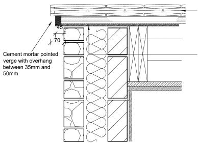
Approved roof covering with tile and half coursing tiles, on top of treated softwood roofing battens to manufacturers specification on top of a Bituminous 1F type roofing underlay and air permeable roofing/breather membrane
