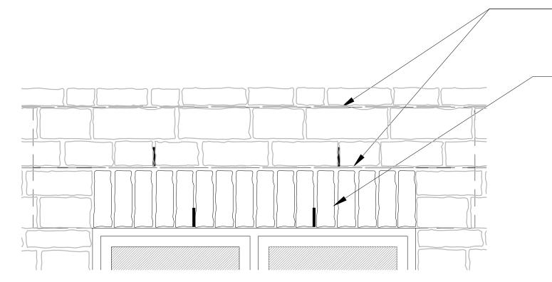
Inner leaf Blockwork reinforcement shown - extend 600mm past opening either side.
