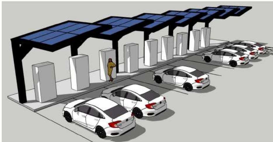
Figure 3: Example image Showing an EV Charge Canopy with PV arrays
