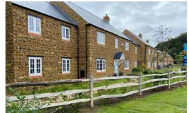
Victoria Park: Variation of building line and roof height to create informal “cottage” appearance.
