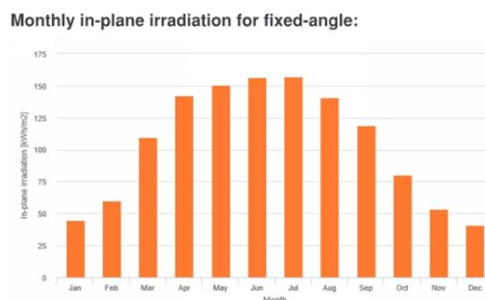
Figure 10: Monthly irradiation for solar PV.
