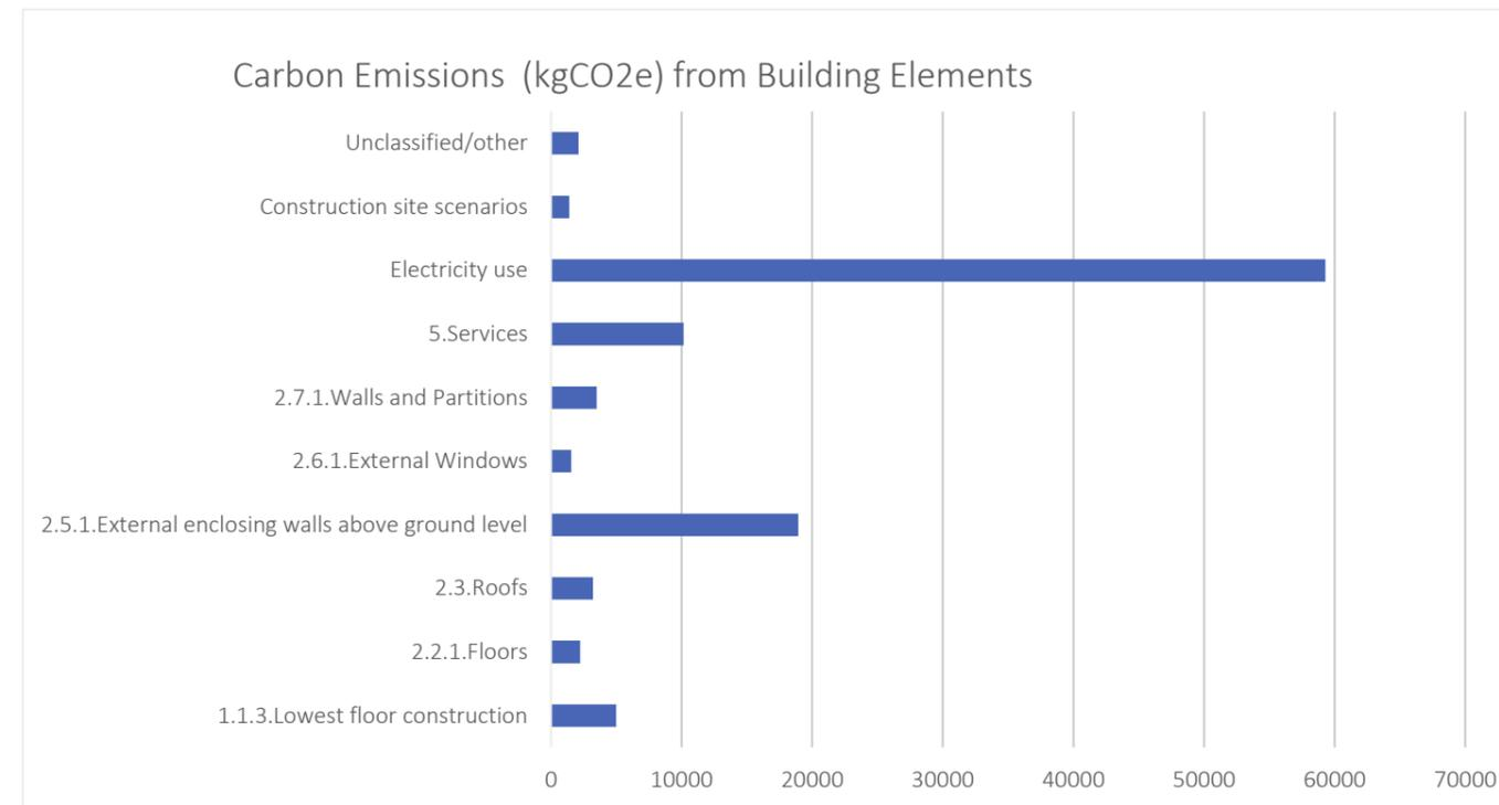
Figure 15 - Carbon emission from building elements
