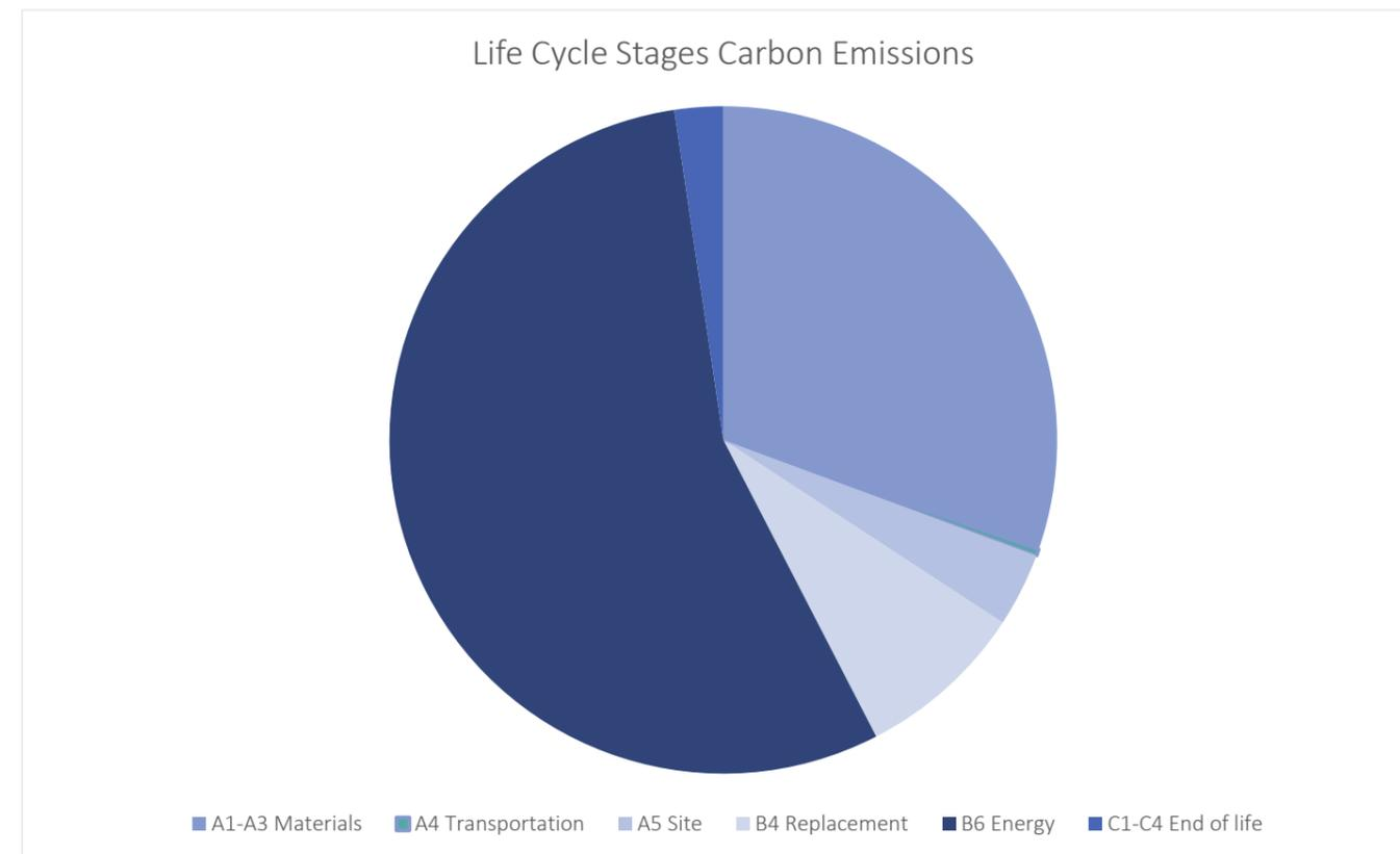
Figure 17 - Life cycle stages carbon emissions
