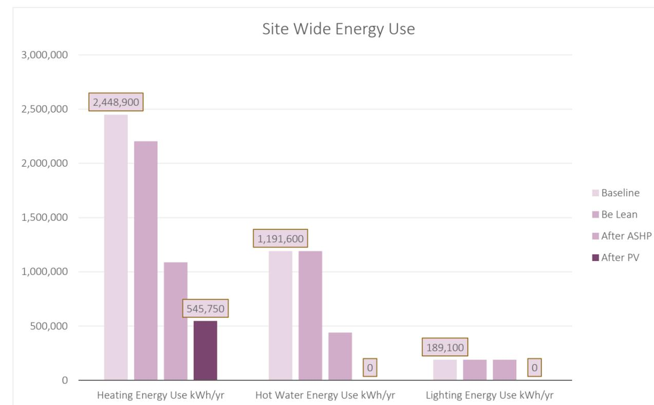
Figure 12 - Site wide energy use after PV (for this calculation PV is assumed to offset lighting, domestic hot water and 50% of the heating demand)
