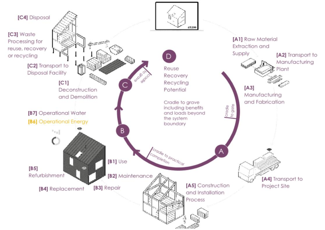
Figure 13 Whole life Carbon Stages (Adapted form LETI Embodied Carbon Primer)
