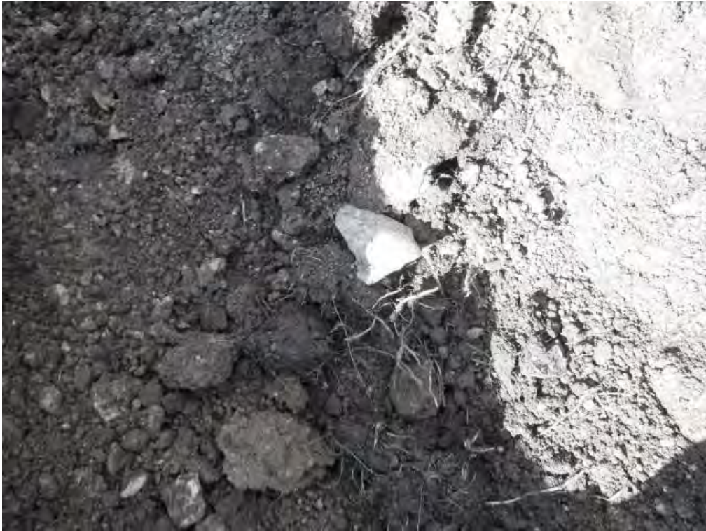
Suspected ACM - Trial Trench TP15
