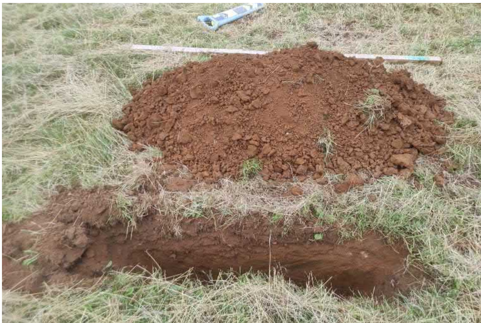
Photograph of arisings from trial pit SA2.
