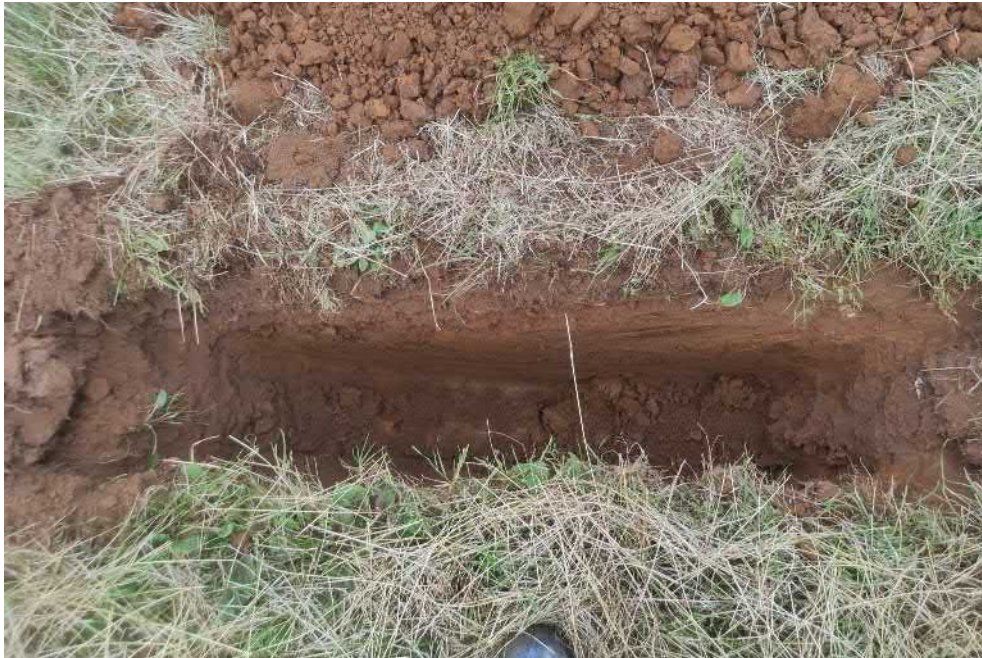
Photograph of trial pit SA2.
