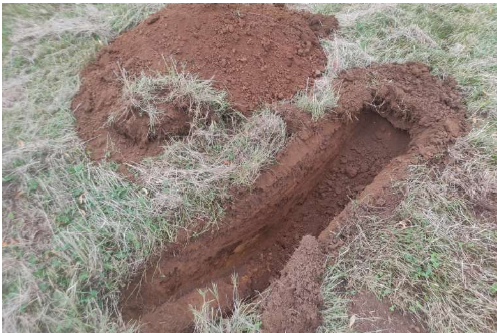
Photograph of arisings from trial pit SA7.
