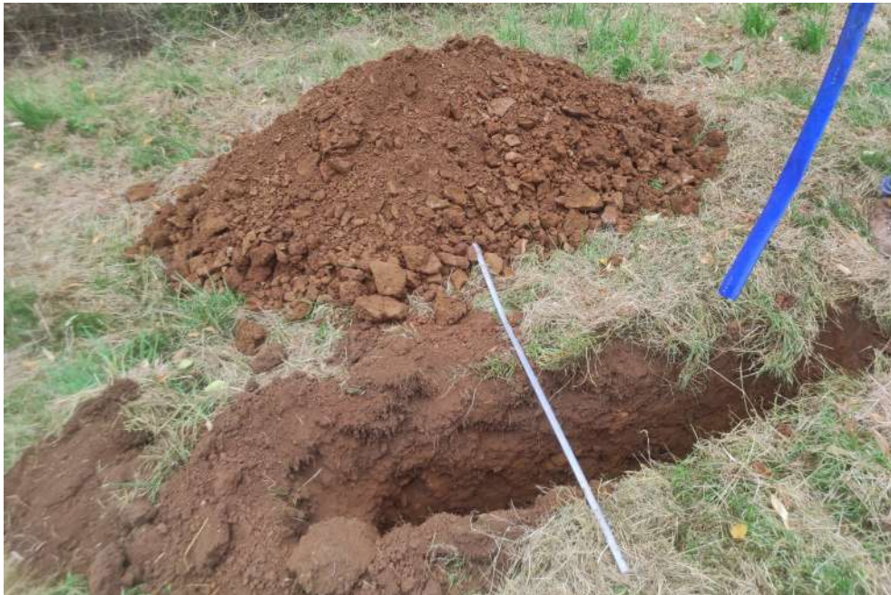
Photograph of arisings from trial pit SA6.
