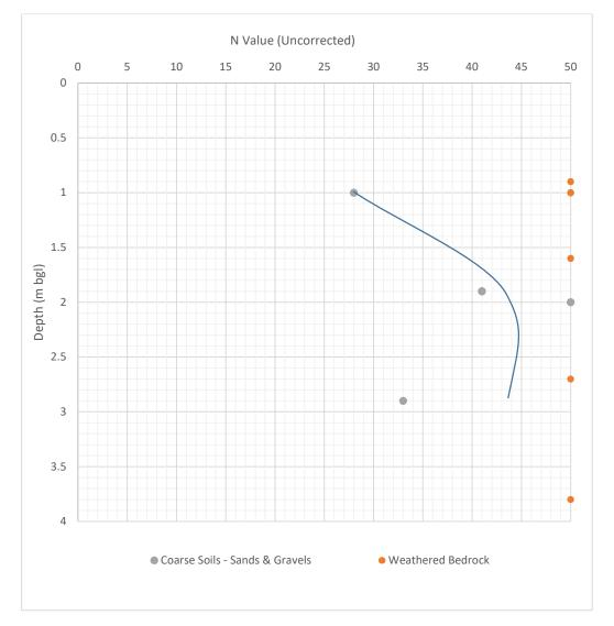
The above graph shows that generally the SPTs were refusing (N Value of 50+) within the granular weathered limestone. The coarse soils denoted in the graph above include the sand layer present at shallow depth and the deeper interbedded gravel layers identified in WS02 and WS07.
