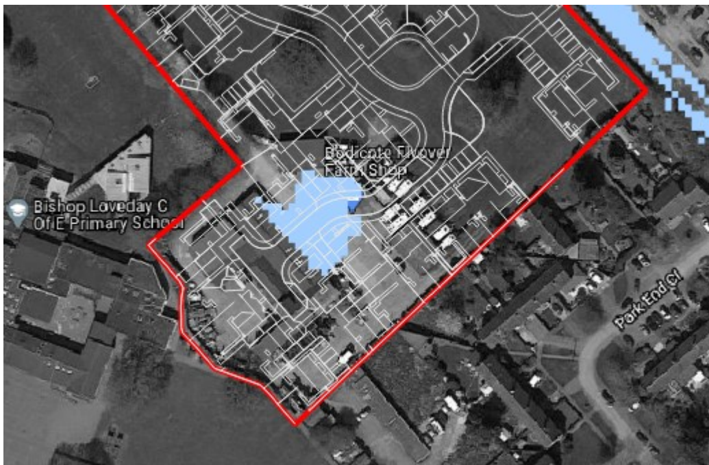
Figure 5. Local Low Risk of Flooding from Surface Water
