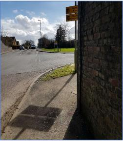
The relocation of the give way line back into Howes Lane means that inter-visibility between a pedestrian waiting at the existing crossing point on the western side and a driver turning left from Howes Lane will be further restricted (existing inter-visibility between users is poor). This may lead to an increased likelihood of pedestrian to vehicle collisions.
