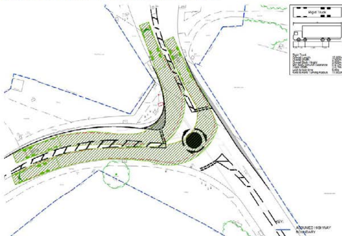
Figure 3-2: Proposed Mini-roundabout Arrangement Swept Path Analysis
