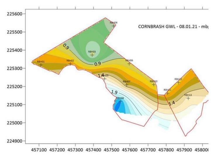
The ground investigation concluded that infiltration is sporadic across the site, with the same geological units being highly variable in infiltration rates, and as such the effectiveness of any single infiltration feature will be highly variable and should not be adopted at the site.
