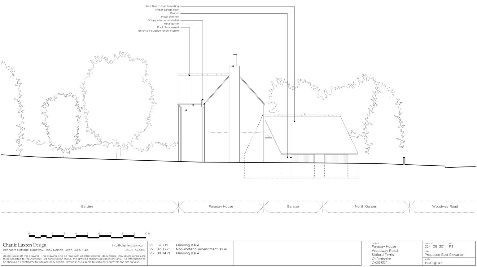
All levels and dimensions to be site surveyed and confirmed by the contractor. See also architectural details, mechanical and electrical intent layout and structural engineers drawings and specifications. Door and windows manufacturer to produce shop drawings for comment before manufacture. All details are intent only, to be finalised by the contractor. Drawings subject to charter approach statutory approvals.
