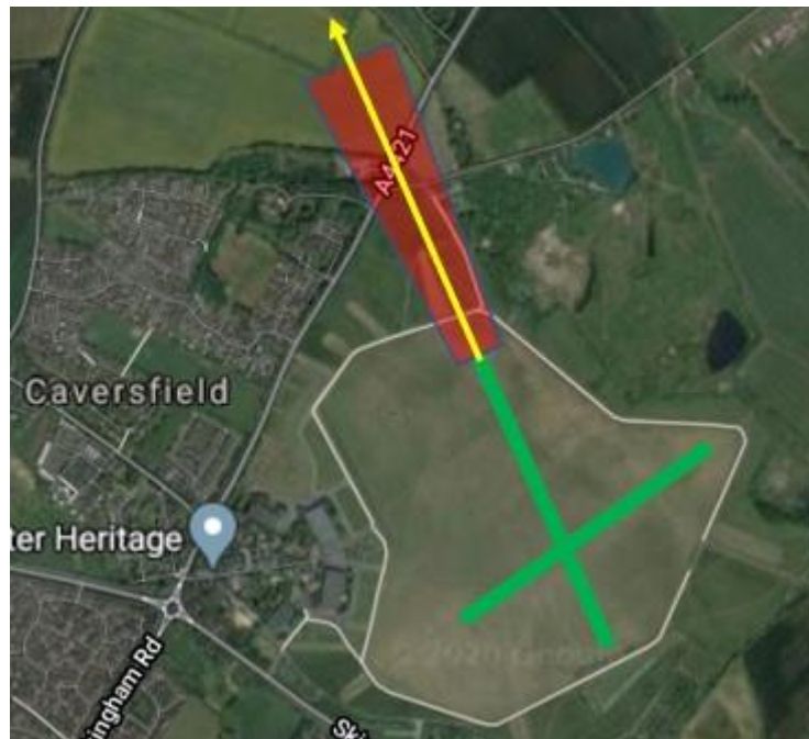
Figure 4.1.3.1. Runway 34 take-off flight path, with a suitable emergency landing area highlighted in red.
