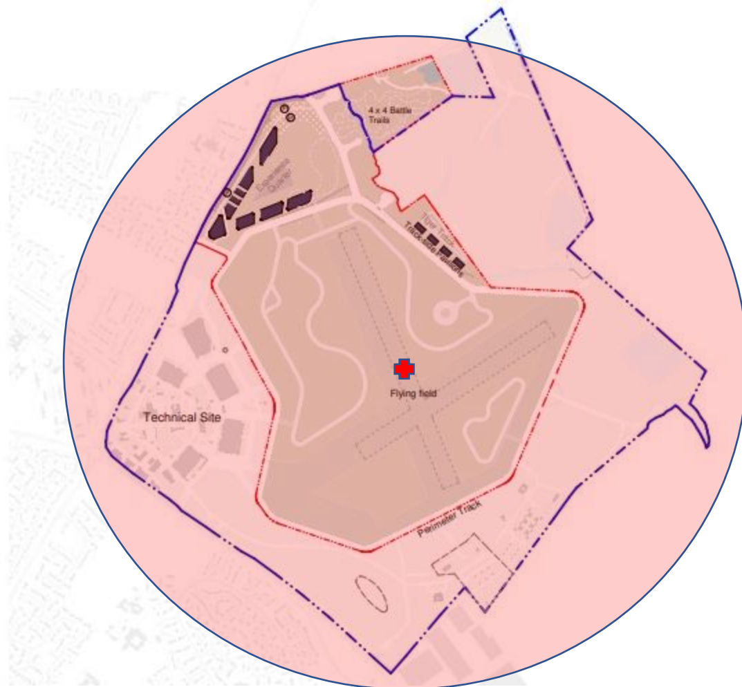
Figure 3.10.4.2. The inner horizontal surface has been surveyed by Ridge to a radii of at least 1000m. The highest noted obstacles are the 'C type' hangars on the aerodrome at a maximum of \leq 20\text{m} .
