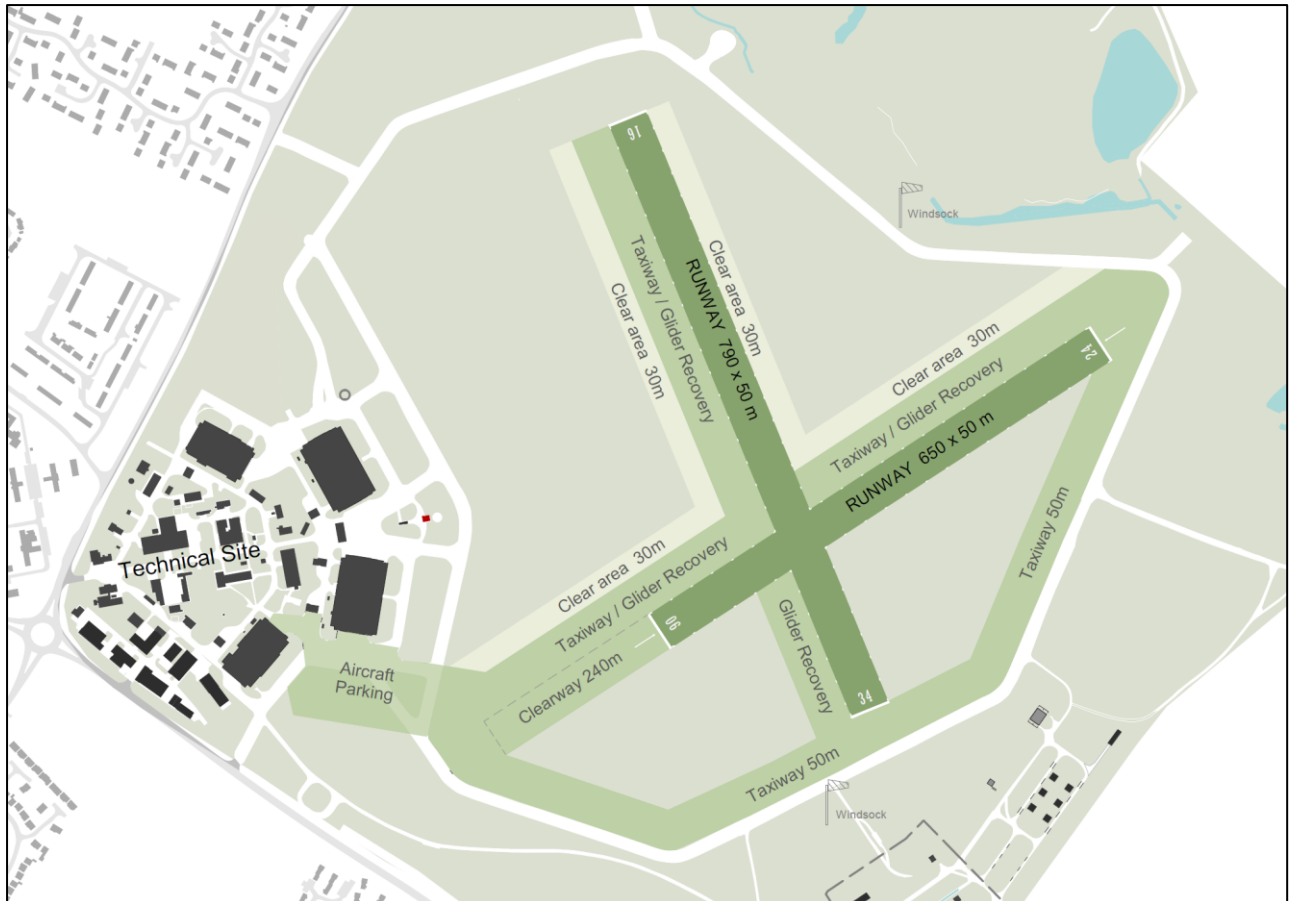
Figure 3.3.1 The aerodrome runway layout and manoeuvring areas
