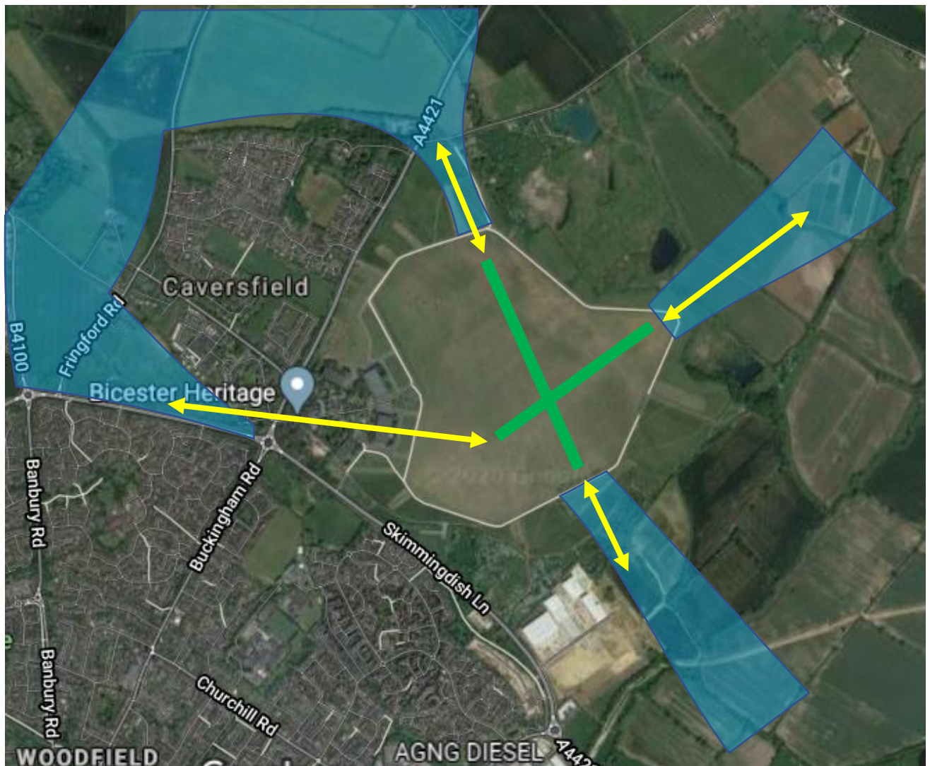
Figure 4.2.1.1 An aerial view of Bicester Aerodrome with appropriate aviation safeguarding areas highlighted in blue. These would allow for relatively low overflight during the take-off-climb and approach-to-land phases of flight, enhancing safety and reducing noise complaints.
