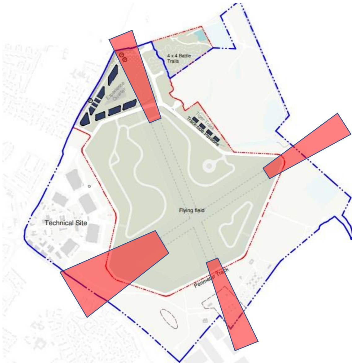
Figure 3.10.6.2 Runway layout with 1:20 gradient take off climb surfaces, and the approach surfaces, highlighted in red, diverging by 10%, with a minimum inner end width of 60m.
