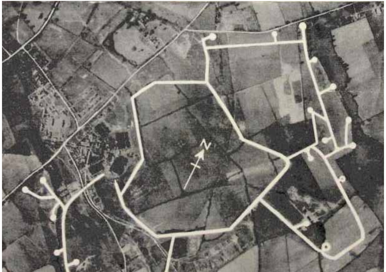
A3: Fig 4. Aerial Photograph of the camouflage scheme at Bicester. Bicester is noted as having been instrumental in the development of aerodrome and camouflage. The aerial photograph illustrates how paint was used to mimic the random shapes field patterns. Camouflage paint was also used on the hangars. The lack of concrete runways and tracks (the latter added c1939) contributed to the success of the scheme.
