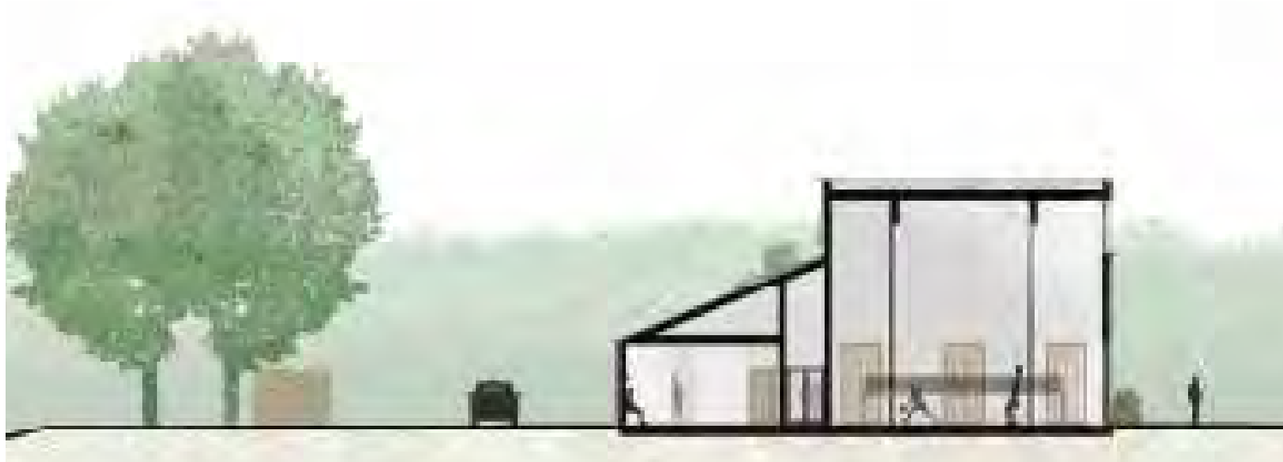
Fig 19: Cross section showing general arrangement and hierarchy of spaces and clerestory / lantern
