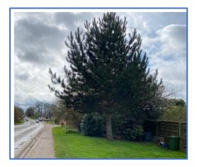
It is acknowledged that a 120m visibility splay has been shown on the drawing. However, there are some large bushes within the verge area and vehicles parked in the existing layby may restrict visibility for drivers emerging from the access. Restricted visibility may lead to pull-out type collisions.
