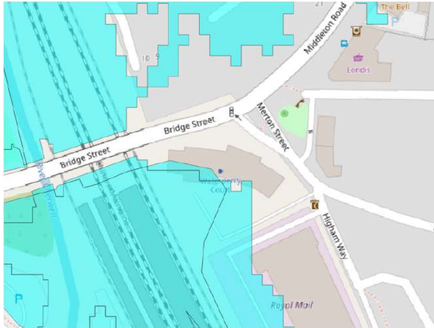
Figure 3: Site location relative to flood zone 2, an area with a greater than 1 in 1000 annual probability of flooding in any one year (Source: EA online flood data).
