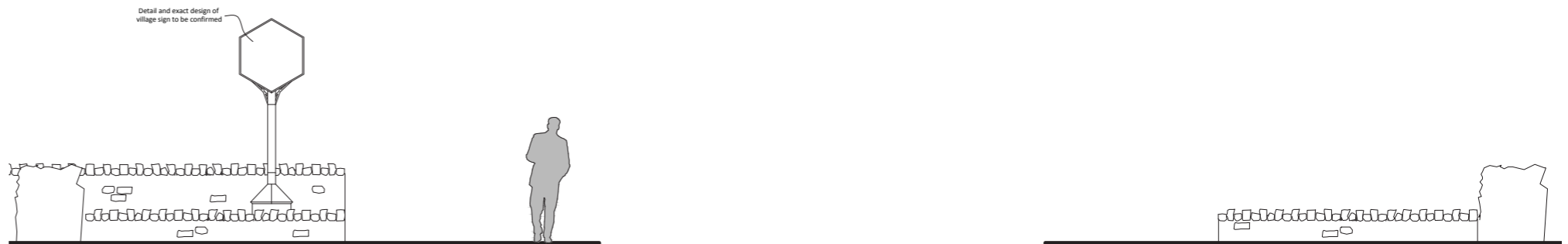
Proposed new entrance gate to site and planters within verge either side of the road to mark the entrance to the Conservation Area
