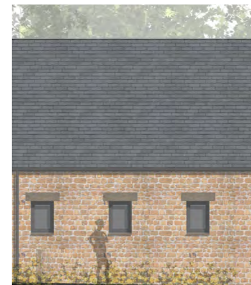
Ventilation Slot Windows
