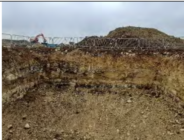
28.04.21 – No visual or olfactory evidence of contamination with PID <0.1ppm in all instances
