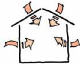
Thermal Bridges use Accredited Construction Details or achieve \psi -value of 0.08W/m 2 K or less
