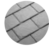
Slates Any variety of natural slate or med/dark grey fibre cement slate
