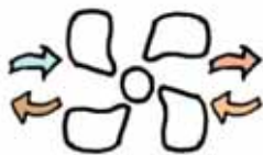
MVHR Efficiencies electrical of 1.5 W/l.s or less heat recovery of 70% or more
