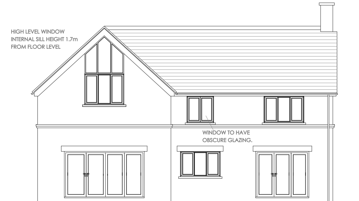
SOUTH WEST ELEVATION
