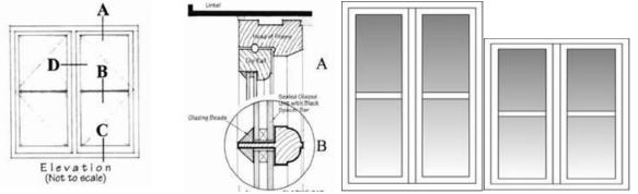
The detail of the glazing bar looks too chunky for the property as it looks to be the same thickness as the casement, it should be 25mm or less. Compare with the elevation on the detail drg which is thinner.
