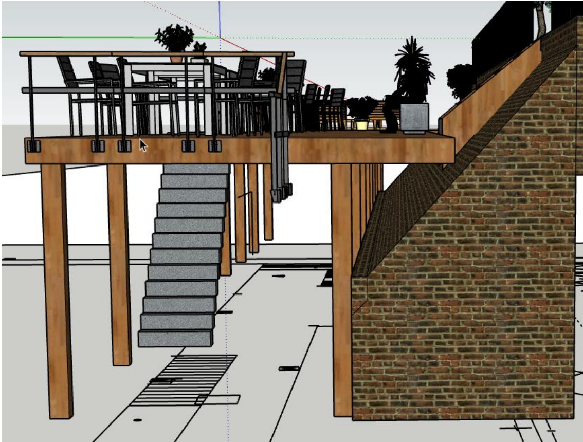
Further images of the proposed Mezzanine decking (Wooden decking with steel sub frame: Currently rendered as wood but will be painted black)
