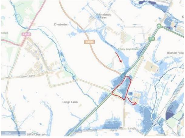
The provided survey shows the ordinary watercourse. This discharges into culvert part way across the site. No mention of culverting of watercourse in FRA for which it will be necessary to seek permission for and easements.
