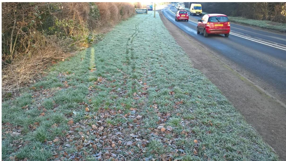
The highway boundary along this stretch is in the grass close to the back of the footway, so the area occupied by the layby and footway/cycletrack will need to be dedicated as highway. The works will be agreed and carried out under a S278 agreement. It is not proposed to have a southbound stop due to the lack of space on the other side of the A4260, but one may be introduced nearby, possibly in the existing layby, at a later date when the Longford Park Phase 2 is delivered.
