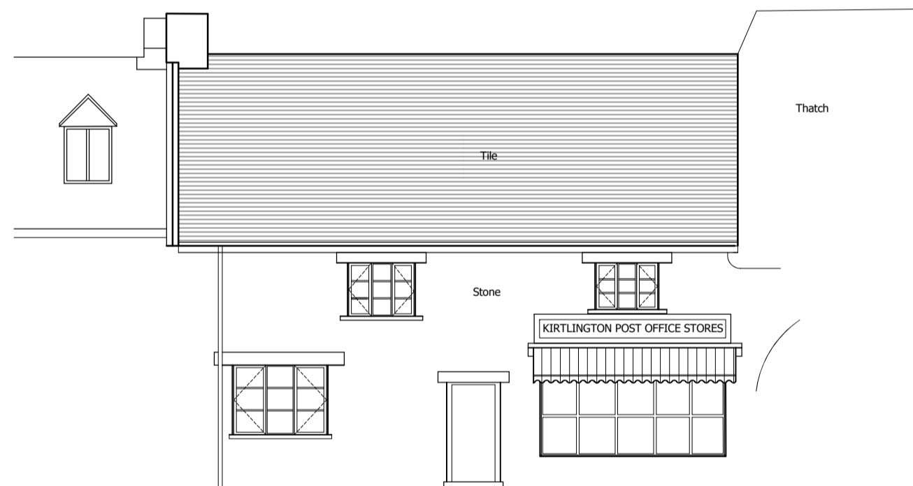
West Elevation (Front) As Existing 1:100@A1
